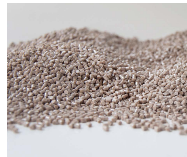
High thermal and chemical resistance: Evonik's VESTAKEEP brand of PEEK polymers.
