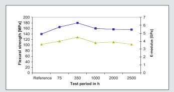
The material excels by its extreme resistance to hydrolysis. The graph shows the mechanical properties of TECAPEEK Classix over stress periods of differing length (hot steam at 200 °C and 14 bar pressure).
